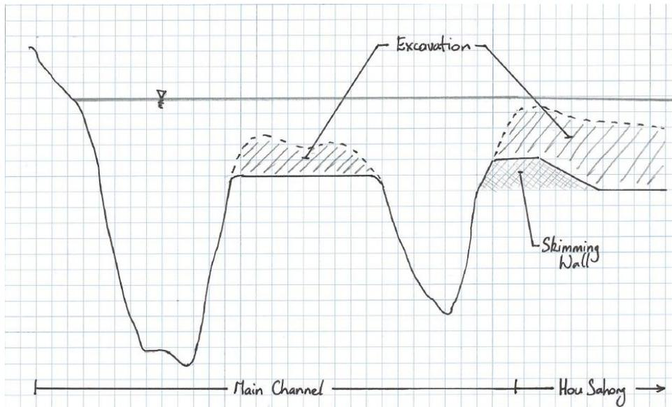
It is expected that the skimming wall will alter the assumed particle size distribution of sediments entering the Hou Sahong headpond (estimated in Section 4.2.1), and so reduce the base-case trapping efficiency estimated (Section 4.3.3) and the corresponding estimated deposition volumes.
