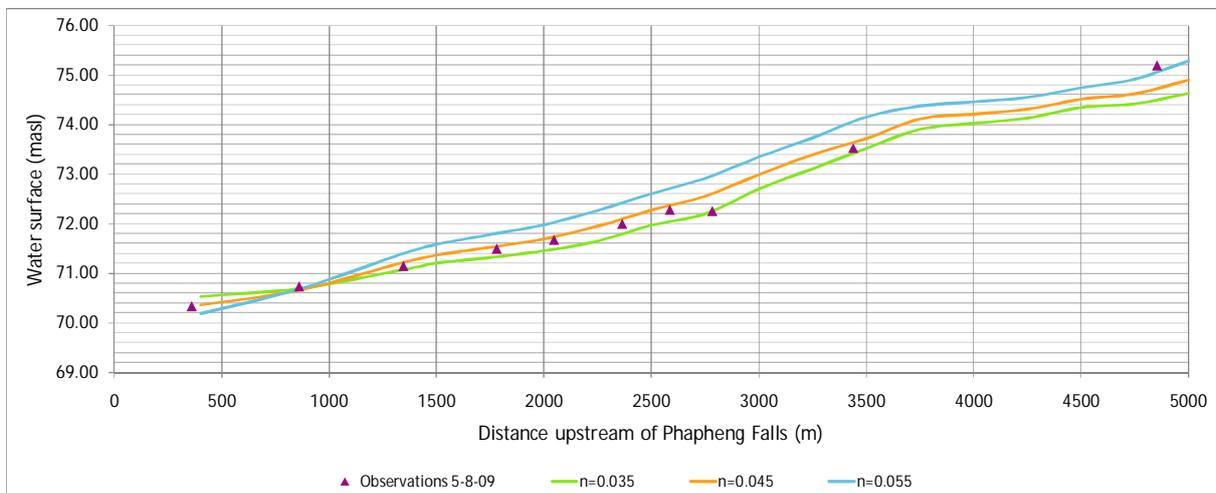
Water-surface observations of 1<sup>st</sup> June 2009 on the right-bank of the Eastern channel are presented in Figure 3-5, together with model results for three different roughness values ( $n= 0.035, 0.045, 0.055$ ). It can be seen that for this flow condition the model results with roughness  $n=0.035$  most closely match observations.
