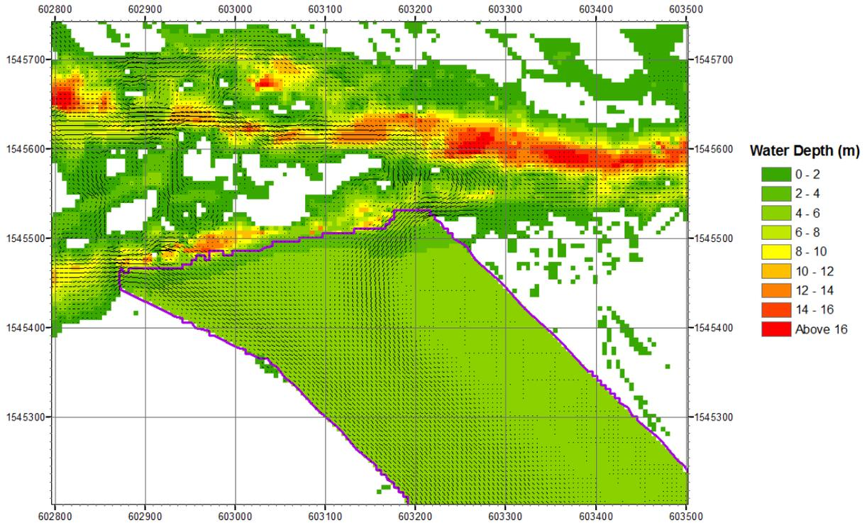
Figure 3-12 shows the results of the proposed Base Case excavation with  $1\ 600\text{m}^3/\text{s}$  diverted, showing a relatively uniform conveyance of flow from the northern channel and into Hou Sahong. The detailed excavation shaping to most efficiently divert flow into Hou Sahong will be determined by the Civil Works Contractor.
