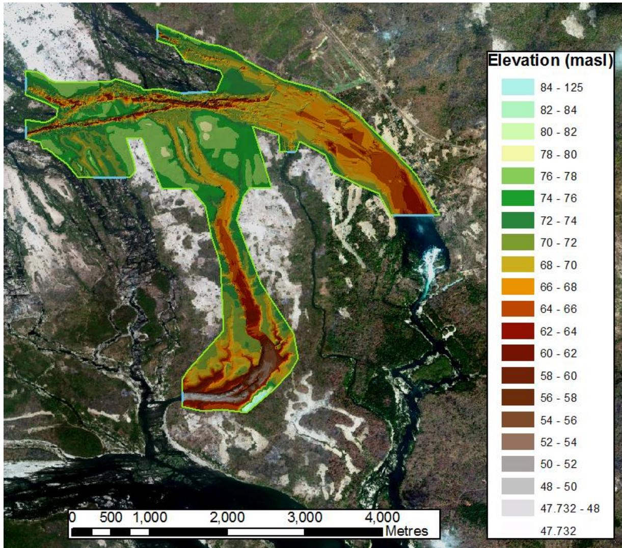
The boundary conditions to the model include four inflow boundaries, 'Hou En', 'Mainstream', 'North1' and 'North2', outflow boundaries for Hou XangPeuk, Hou Sahong / powerhouse, and Hou Sadam, and a defined water surface at the downstream Eastern Channel boundary.
