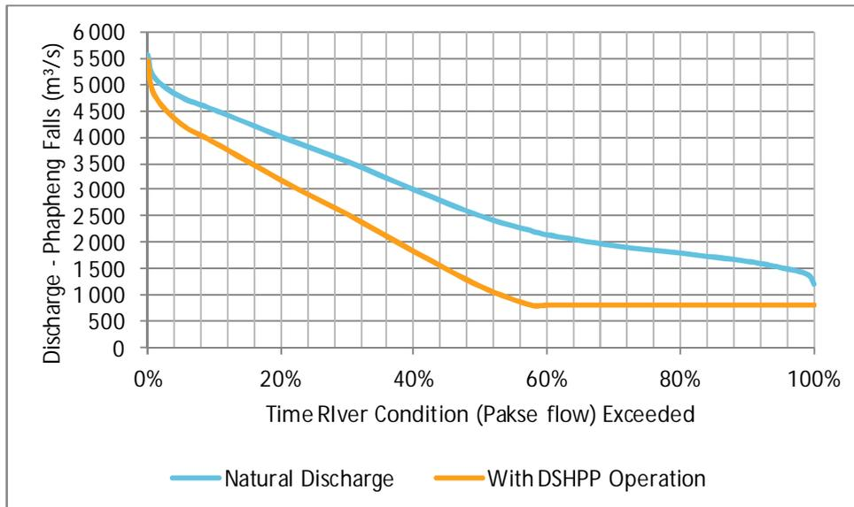
The reduced flow over Phapheng Falls will result in lower water levels at the Hou Sadam inlet. Excavation is planned at the inlet of the Hou Sadam, to encourage fish migration, with the intention that the flowrates in Hou Sadam with DSHPP in operation will match the natural flowrates for the same river conditions. The current modeling assumes the same flowrates in the natural and developed conditions, and includes excavated bathymetry to provide this.
