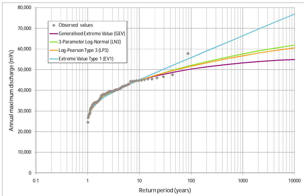
The maximum observed annual peak (57 800 m<sup>3</sup>/s in 1978) is significantly higher than any other in the 87 years of record. The EV1 distribution closely fits this point but over-predicts more frequent floods, for example predicting a 1/20 AEP flood of 48 000 m<sup>3</sup>/s which was only exceeded once (the 1978 flood) in the 87 year record.
