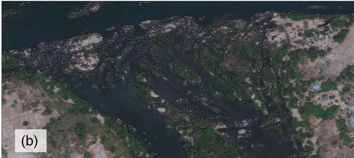
Water-surface observations of 5<sup>th</sup> August 2009 on the Eastern Channel are presented in Figure 3-4, together with model results using three different roughness values ( $n= 0.035, 0.045, 0.055$ ). It can be seen that the model results with roughness  $n=0.045$  most closely match observations. The most upstream observation is at discharge gauging location CS02, approximately 600m upstream of Hou Sahong inlet.
