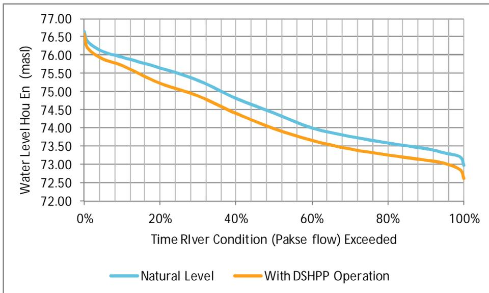
Water levels within the Hou Sahong headpond will be substantially increased over their natural levels in the mid and downstream sections, due to the presence of the dam.
