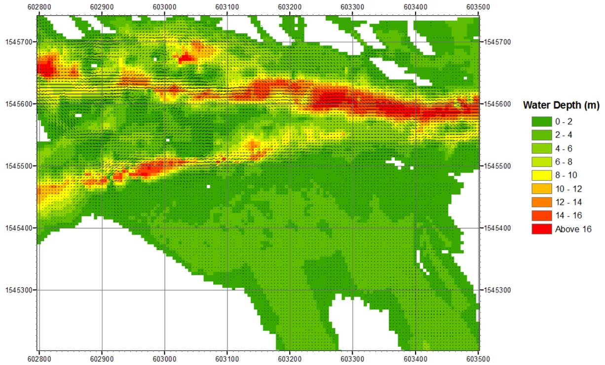
**Figure 3-11: Flow depths and velocities modelled at Hou Sahong inlet for station operation with Hou Sahong excavation but no excavation to the reef at eastern tip of Don Puay,  $Q_{Pakse}=4\ 734\text{m}^3/\text{s}$ ,  $Q_{Sahong}=1\ 450\text{m}^3/\text{s}$ . Outline of excavated area is shown.**
