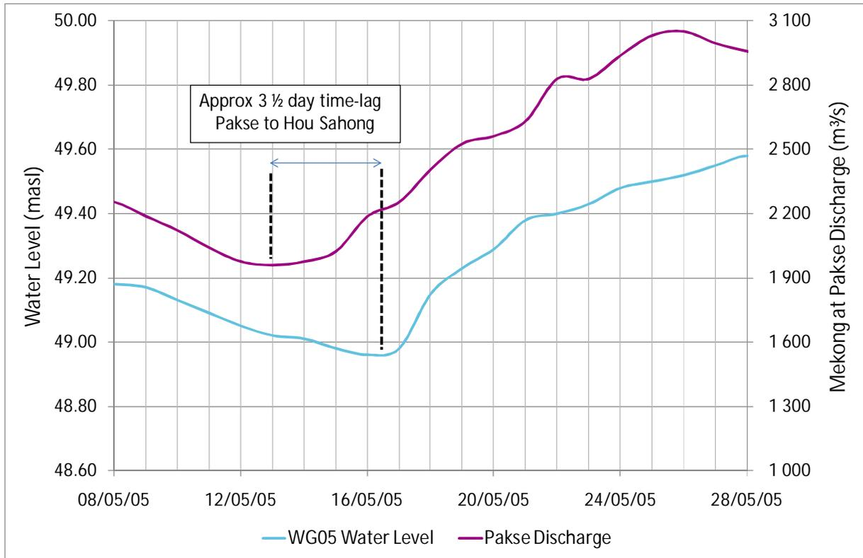
Estimates of time lag can be analytically achieved using a simple kinematic wave model, assuming a wide channel of constant depth between Pakse and the site. This model agrees well with gauge-board observations (e.g. Figures 2-7 and 2-8).
