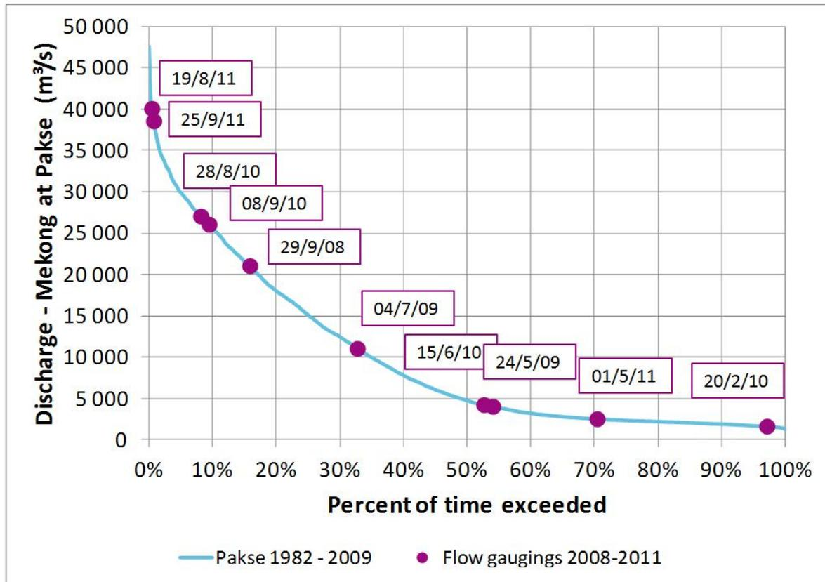
A further flow gauging exercise was completed by contractors ASA Power in May 2011. The flow measurements, carried out using a Price AA current meter, were principally to provide medium-low flow measurements in conditions where ADCP measurements were difficult. The results are tabulated below.
