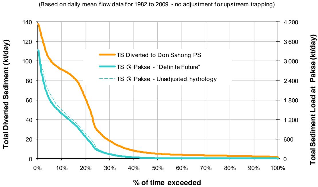
Figure 4-8: Duration Curve of Total Sediment Concentration Diverted to Headpond.
