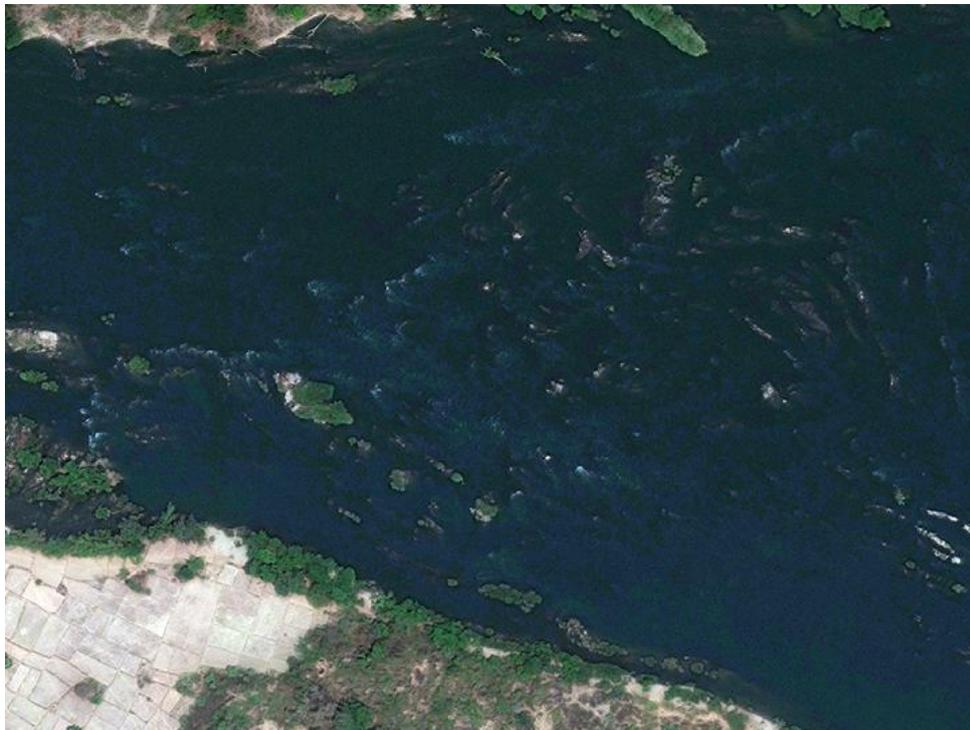
Figure 3-8: Flow in Eastern Channel reaching vegetation canopies during high-flow conditions, 25-9-10,  $Q_{Pakse}$  23 000 m<sup>3</sup>/s.
