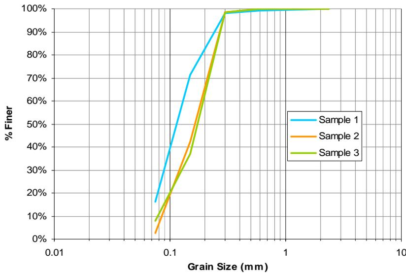
Figure 4-2 indicates that sediments deposited on the river beaches are generally in the fine sand range, mostly between 0.075mm and 0.3mm, with a maximum size of about 0.6mm. It is not possible from these samples to identify the proportion of the total transported sediment that these sands make up. However it is apparent that they represent the largest sizes transported by this reach of the river.
