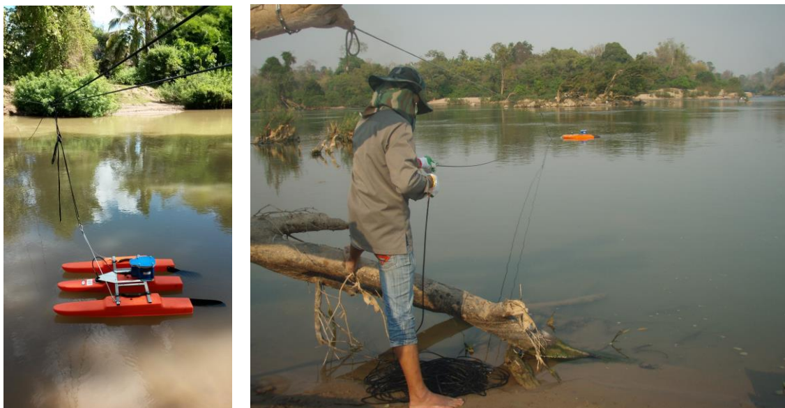
Figure 3-12: Teledyne RDI 'StreamPro' ADCP
