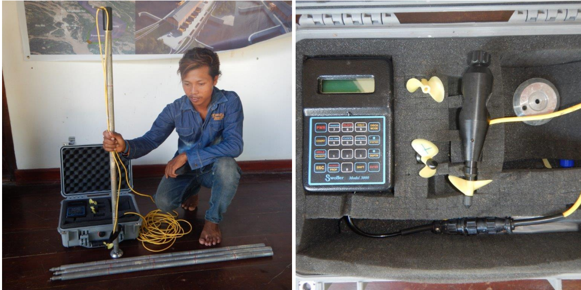
Figure 3-14: Swoffer 3000 current meter used for supplementary flow measurements
