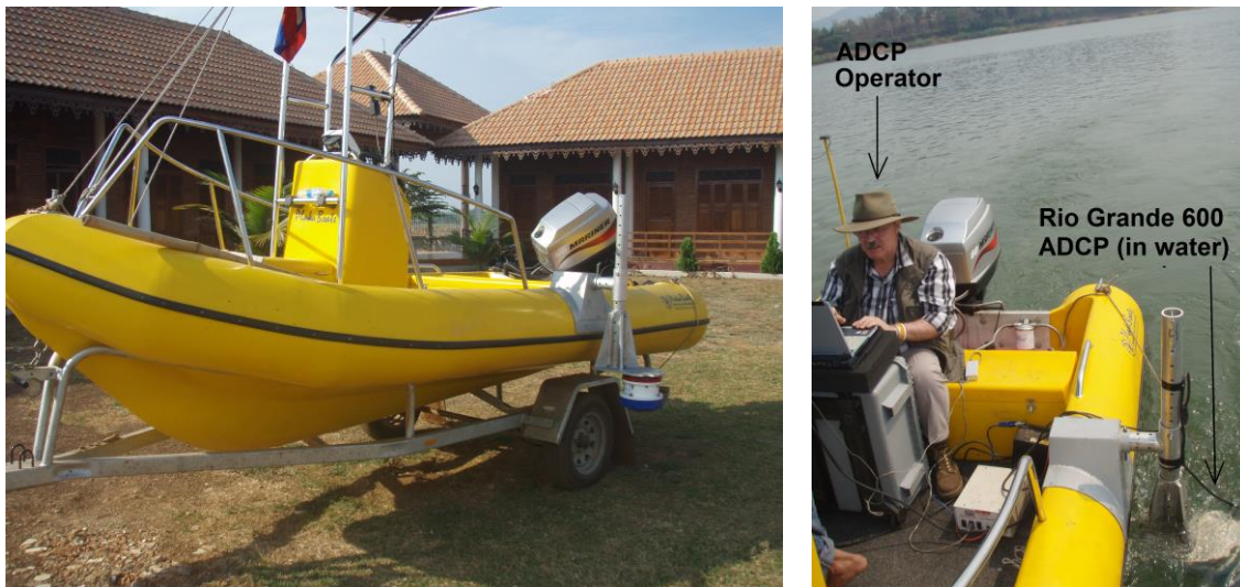
Figure 3-11: Teledyne RDI Rio Grande 600 ADCP mounted on 4.6m polyethylene Plaka boat
