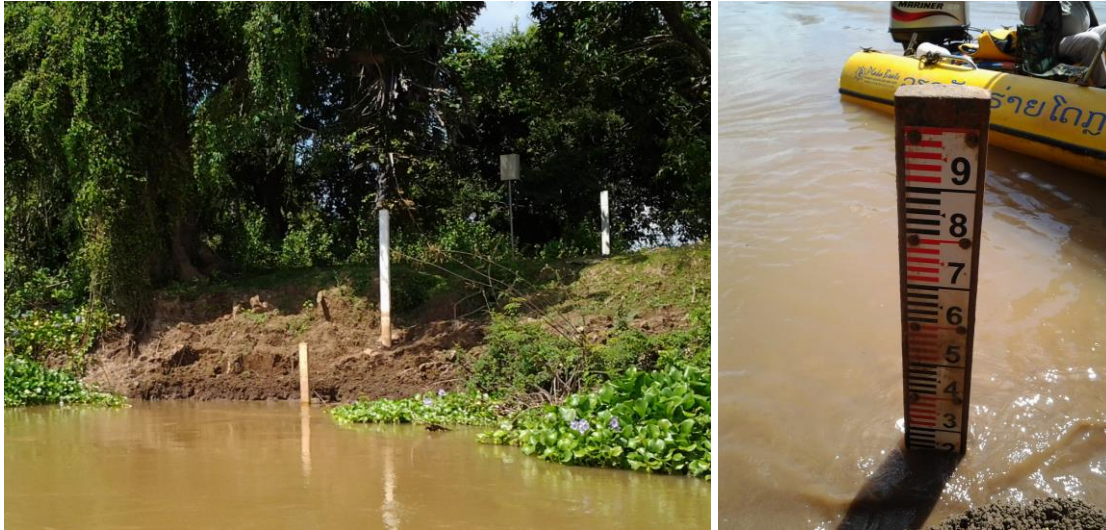
Figure 3-16: Staff gauge boards at AR01
