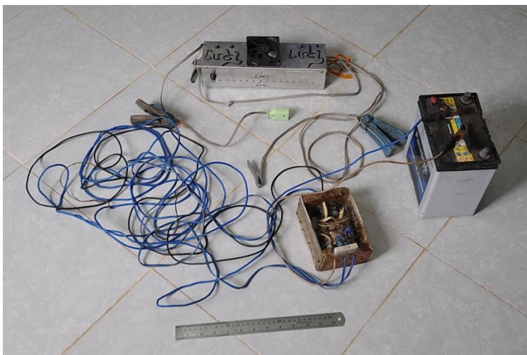
Figure 10 Two battery-powered electrofishers held at Khong District office of PAFO
